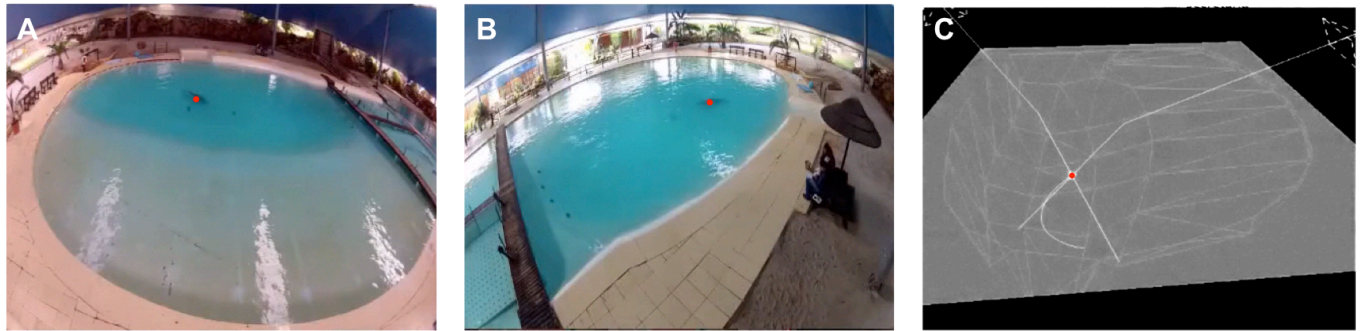
Figure 2.7. Three-dimensional reconstruction of the pool. A – Image from the entrance camera showing the dolphin and the red dot from the tracking recognition. B - Image from the second camera showing the dolphin in the same frame as image A, and the red dot representing the centroid of the animal. C – Three-dimensional reconstruction of the pool using the algorithm. The two vectors are going from the two cameras to the dolphin (intersection of both vectors) giving the 3D position of the animal in the pool (red dot).
