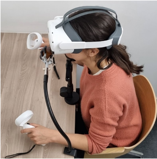
Fig. 3. The experimental setup. Participants were asked to wear a virtual-reality headset and place their chin on a chin rest. A metal claw held the vial containing the super-donor sample 2 cm away from the participants' noses.
