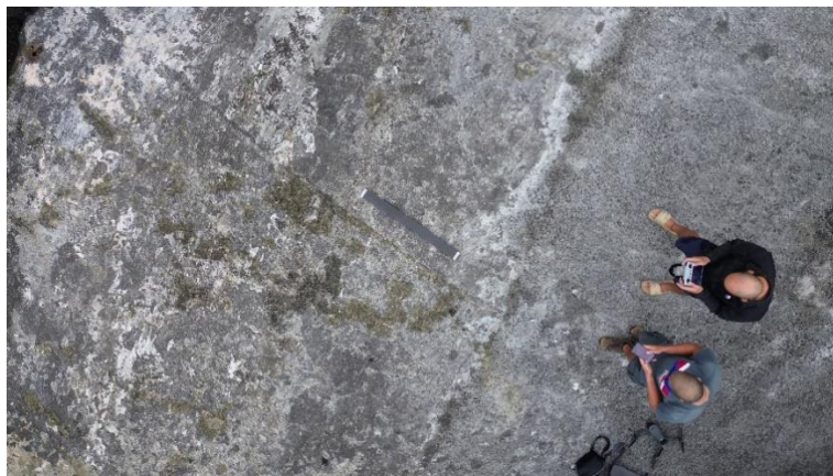
FIGURE 7 – Screenshot of the DJI Mini 3 calibration flight, at 5 m of altitude, with the 100-centimeter-long bar in the centre of the camera field of view.
