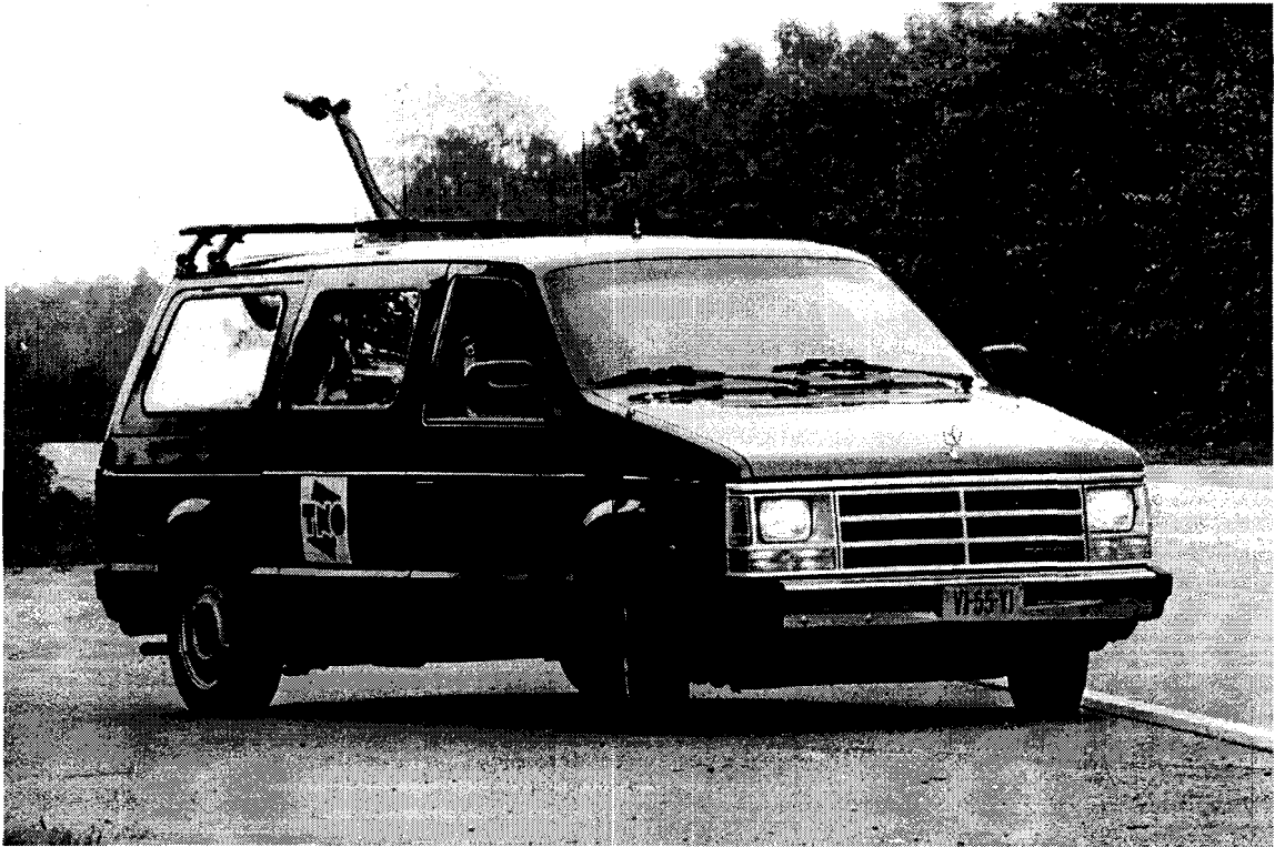
FIGURE 1 Instrumented Car for Computer Aided Driving ICACAD
